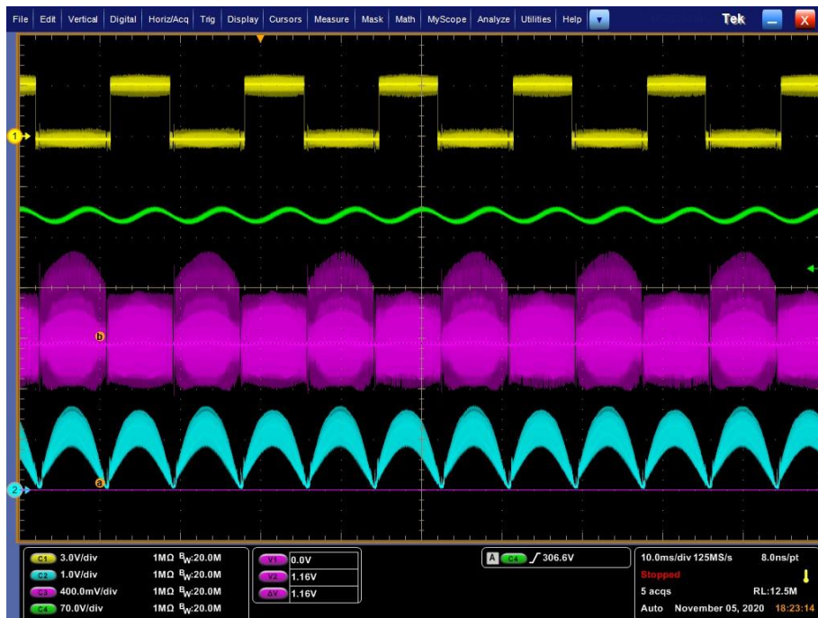
Fig. 15. Additional waveforms obtained from the totem-pole PFC evaluation board with V_{in} = 180 Vac and output power = 500 W.
